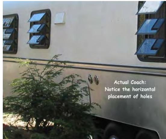
Our extensive study of replacement furnaces told us that the new furnace would use a vertical hole arrangement; therefore, our existing horizontal holes would not be useable. For safety reasons, the manufacturer strongly warns that intake and exhaust tubes NOT be bent or shaped, but should be connected directly to the holes in a straight line. We'll take their advice on that one, too!
