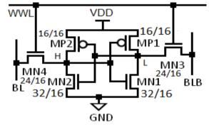
Figure 2: Standard 6T SRAM cell (D6T).
