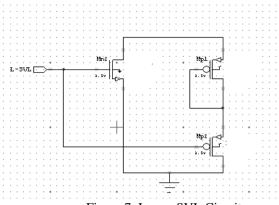
Figure 7: Lower SVL Circuit
