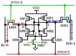
Figure 5: Write Operation of the proposed 8T SRAM cell
