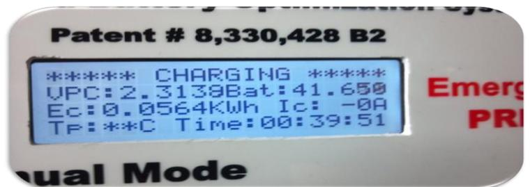
The batteries would then be discharged and the runtime in amp/hours, minutes and KWH would be recorded. Both batteries would then be re-charged and the metrics again recorded, this would then be the baseline performance data. **Note: Since the KWH of both the charging and discharging cycle is measured, the client can for the first time accurately compare the electrical efficiencies of the batteries as a ratio of KWH in and out.**
