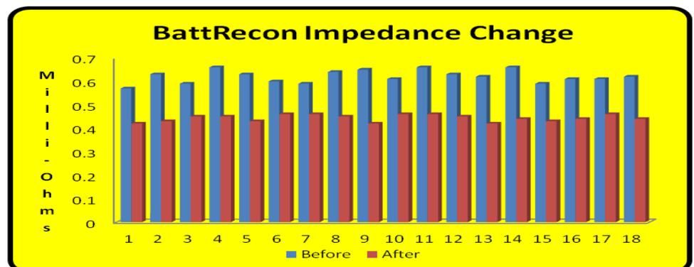
and the results varied from between .55 and .66 milli-ohms per each individual cell. The impedance values were tested by inserting a stainless steel screw into each corresponding cell terminal after which the Kelvin
