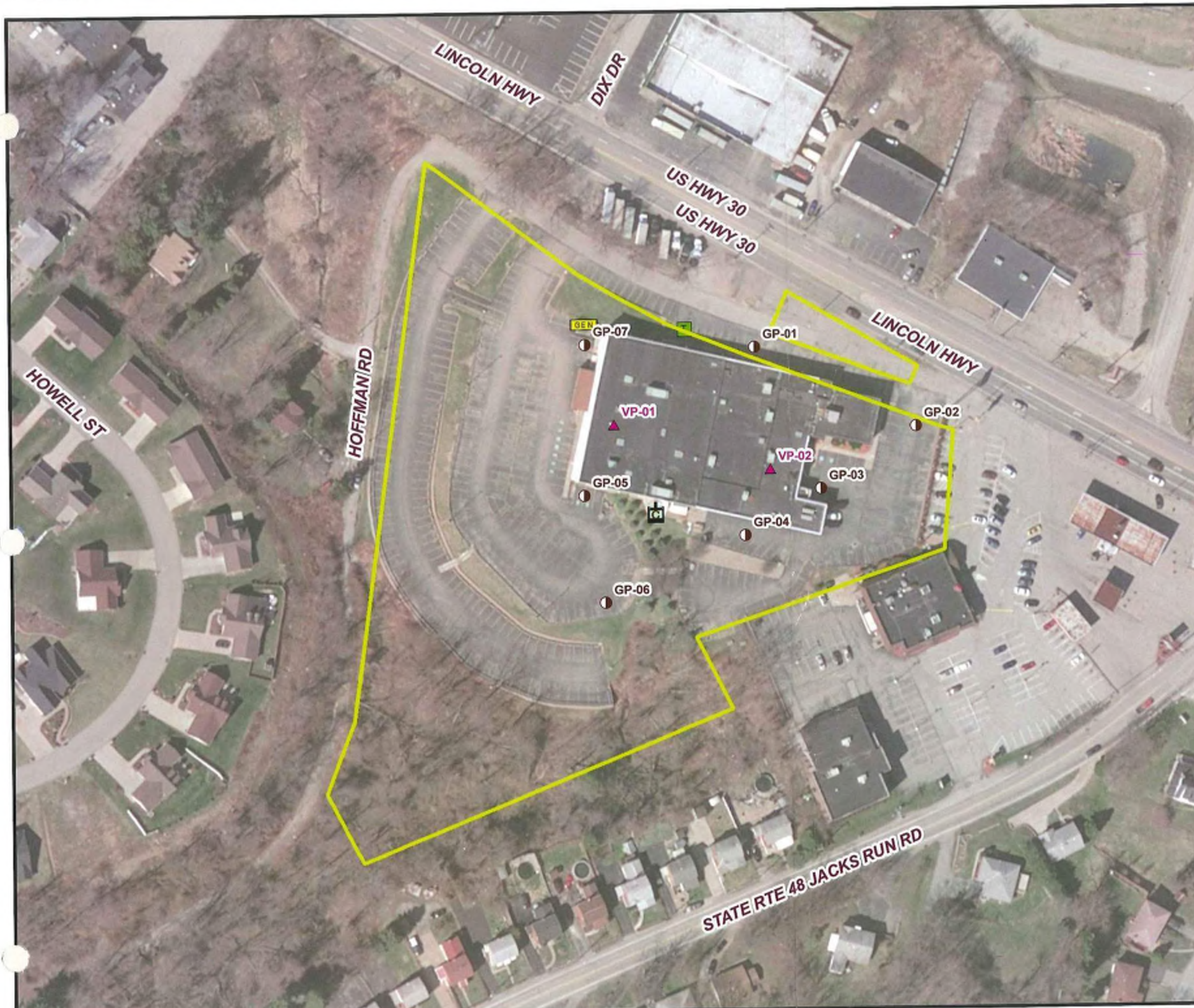
FIGURE 1 SITE LAYOUT AND SAMPLE LOCATIONS PHASE II ENVIRONMENTAL SITE ASSESSMENT LINCOLN HIGHWAY PROPERTY 1810 LINCOLN HIGHWAY NORTH VERSAILLES, ALLEGHENY COUNTY PENNSYLVANIA
