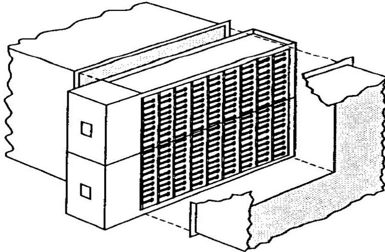
*Two stacked sections in a duct*
