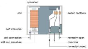
Figure 3: SPDT Internal Structure
