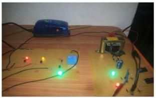
Figure 7: Green LED- Level 3 reached indicating the tank is completely filled
