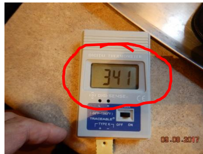
The upper oven heated to 341° when set to 350°.
