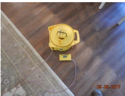
Foundation elevations using digital water level
