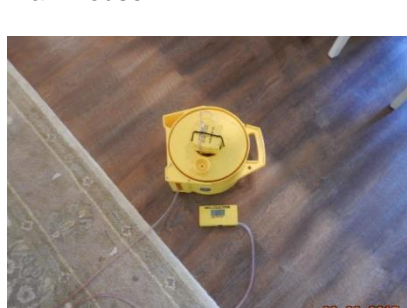
The floor elevations were checked with an electronic digital water level.
