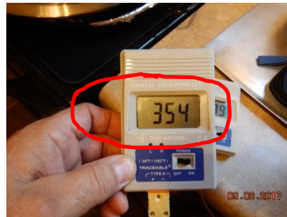
The lower oven heated to 354° when set to 350°.
