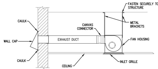
**2 CEILING EXHAUST FAN DETAIL**
