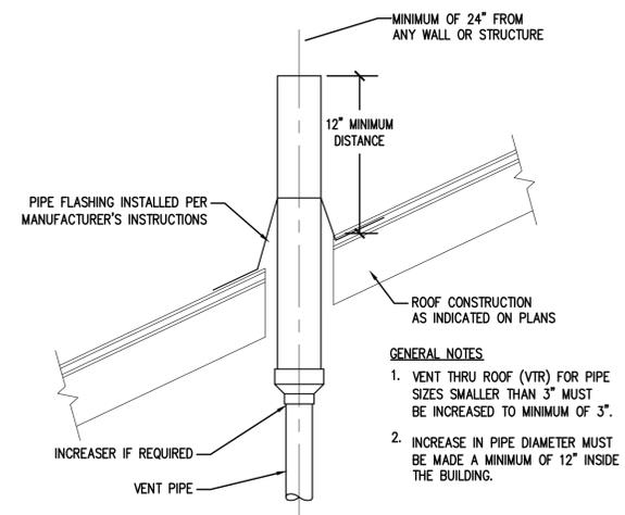
**5 VENT THROUGH ROOF DETAIL**
