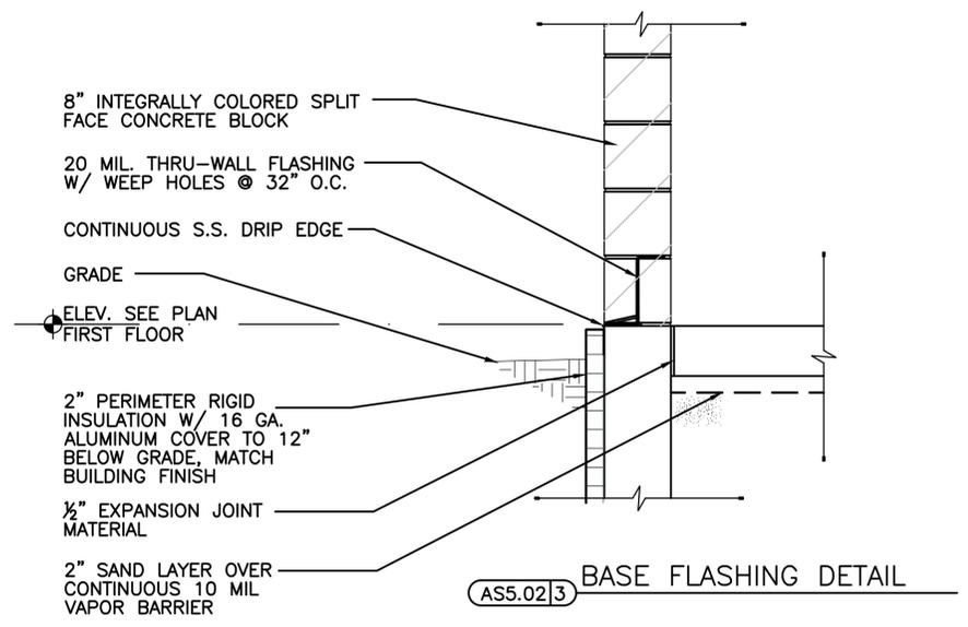
AS5.02|3 BASE FLASHING DETAIL
