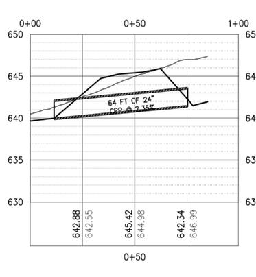
**PROPOSED WATER TANK ROAD CULVERT**
