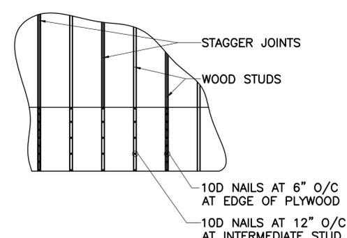
ELEVATION - GABLE WALL NAILING DETAIL
