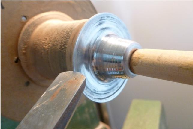
For larger pieces, it will be necessary to trim the edge. Trimming keeps the edge of the piece concentric with its center and relieves some tension that builds up in the piece. The effect is like slightly annealing the piece. When the piece is almost complete, burnishing or polishing the piece is usually done while still mounted on the lathe.
