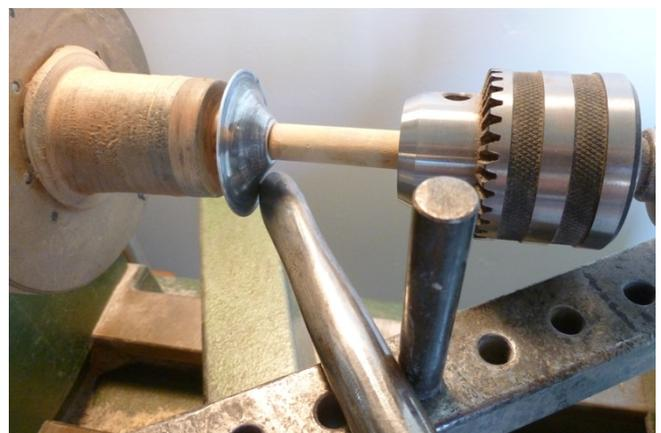
with the metal blank, reducing friction and heat. Typical RPM while spinning is 500-1000. Be sure that the disk is precisely centered. Experienced spinners can do this with the lathe running by loosely holding the disk between the chuck and follower block and centering with a push stick. This is an extremely advanced and dangerous practice so it is advised that you center the disk before starting the lathe.
