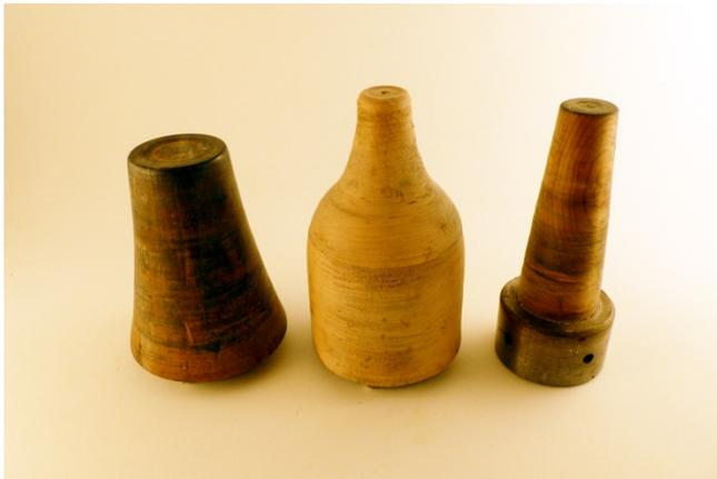
"Chucks" are the positive forms that metal is spun up against to maintain uniformity while producing a series of similar pieces. Most of the spinning of any piece is mostly done "on air" (the metal not up against the chuck). The metal is only spun against the chuck at the end of spinning to help ensure the piece has the required form and dimensions. When making prototypes or one-of-a-kind pieces, any chuck can be used that will not interfere with the final form desired.
