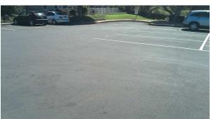
This component is for asphalt overlay and striping of all asphalt. Asphalt can last 25 yrs or longer if seal coated and maintained properly. Asphalt should be seal coated every 5 yrs to protect the base surface from the destructive UV ray. New Asphalt should be seal coated with in the first 2-3 years to protect the base coat.
