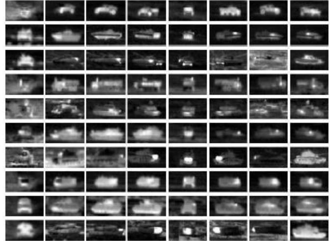
Fig.3: IR chips of 10 targets in 8 orientations in the Comanche database
