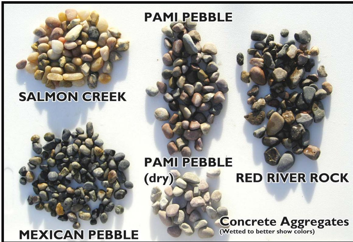
**6- Seeded Aggregate Finish:** Small decorative stones are imbedded into the top layer of concrete, and during the finishing process, exposed to give a pebble texture to the concrete finish. This is a similar technique to exposed concrete, but instead of exposing the natural concrete aggregate, decorative aggregate is added when installed. (Cost \$\$\$)
