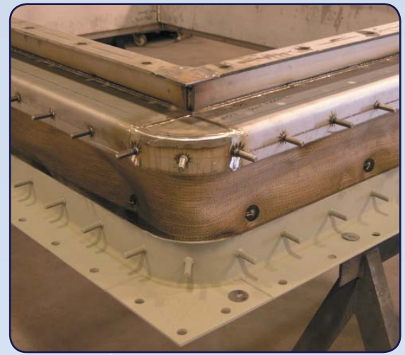
Hot-Cold Rect. GTEJ showing insulation before belt mounting
