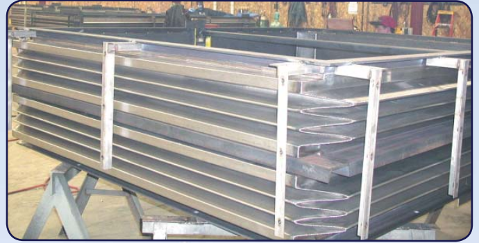
Primary Air FD Fan Duct Expansion Joints
