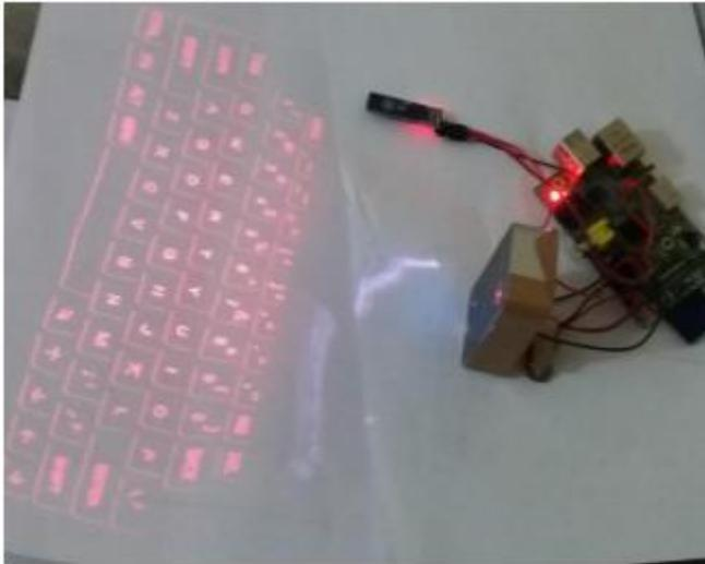
Fig.5: Virtual Keyboard display unit
