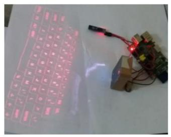
Fig.5: Virtual Keyboard display unit
