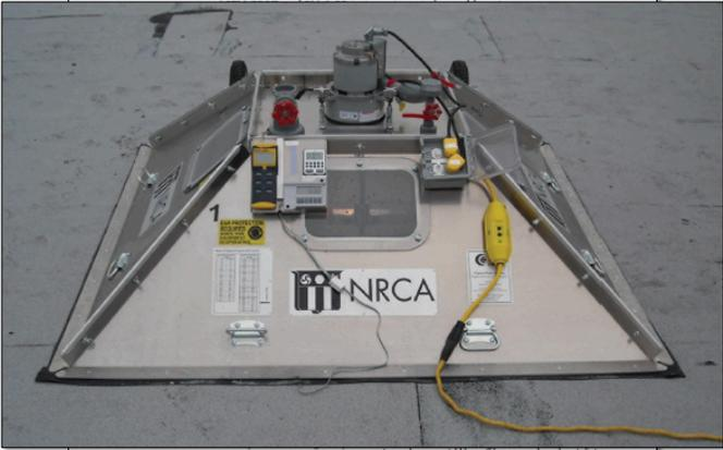
5-foot dome-like chamber to a roof surface's upside and applying a defined negative (uplift) pressure inside the chamber to the roof system's exterior-side surface using a vacuum pump (see photos). During the test, membrane surface deflection inside the chamber is visually monitored and measured to determine whether a roof system passes or is "suspect."
