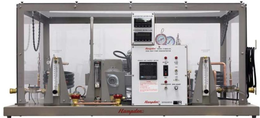
**MODEL H-6820** Dual Heat Pump Demonstrator
