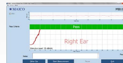
Patented chirp stimulus and advanced response detection algorithm allow fast test times.
