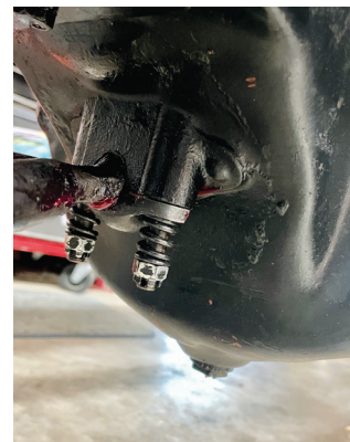
Greased cap in place with springs compressed, castle nuts awaiting safety wiring
