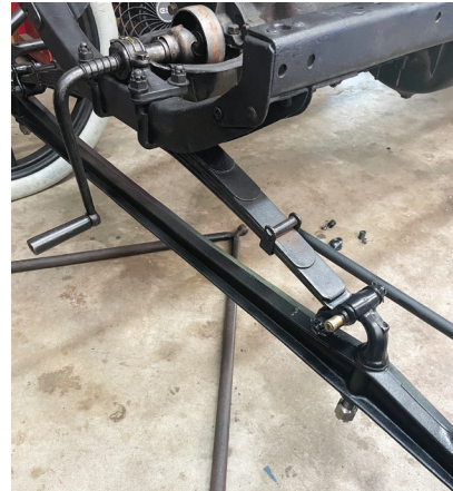
Chassis ready for installing the front axle radius rod
