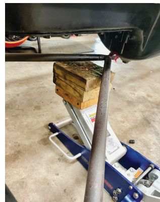
Jack with wood support used to lift the radius rod into the crankcase socket
