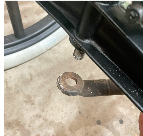
Perch end of radius rod showing round hole, not oblong
