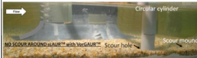
**Example AUR flume test of pier with scAUR™ and VorGAUR™ - NO SCOUR! Note scour on cylinder.**
