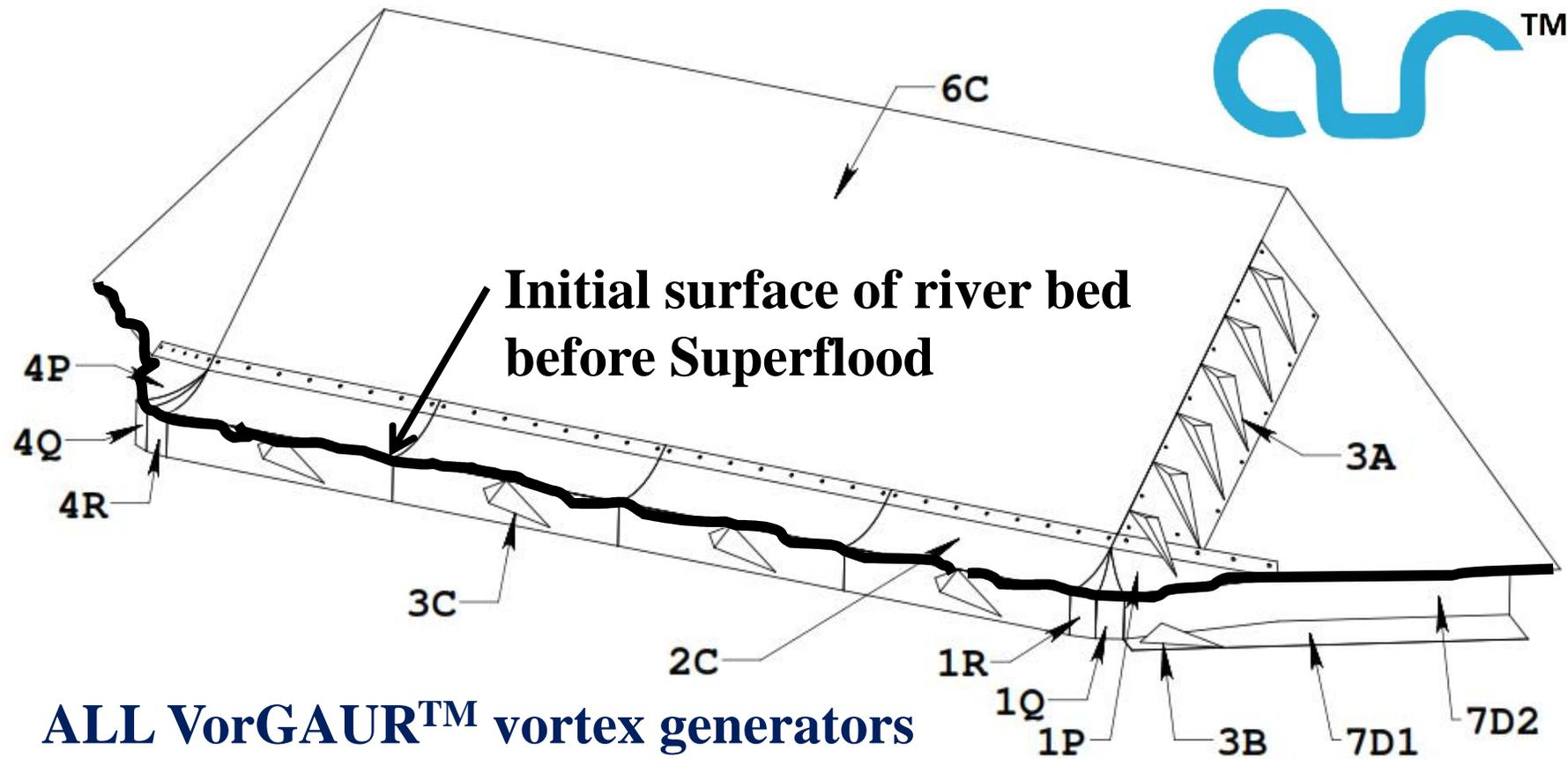
**ALL VorGAUR™ vortex generators produce stream-wise vortices that move up the foundation and wall, bringing river-bed material toward the abutment**
