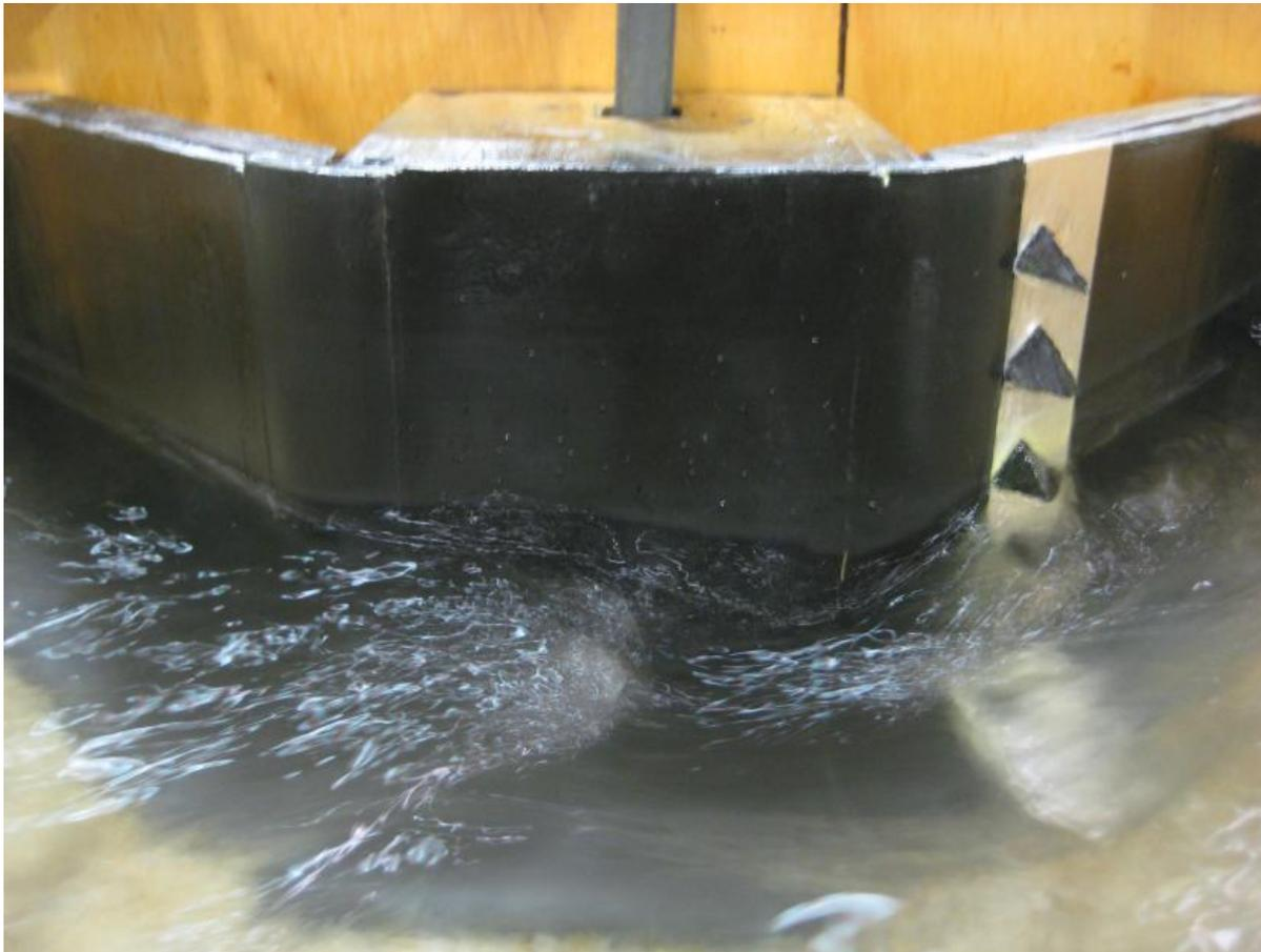
**View of case #20 modified wing-wall abutment model with VGs. Note the free surface height change after the contraction due to the surface vortex.**
