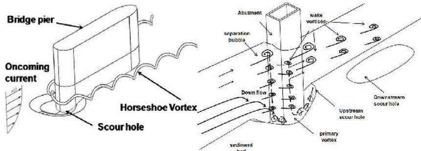
Bridge scour is produced by discrete vortices formed around unprotected piers (left) and abutments (right)
