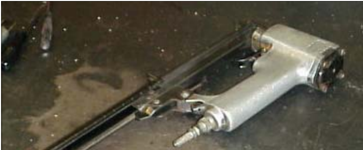
7. Here's the tool to use to staple the cover to the base. It's a pneumatic stapler. If you use an electric stapler or a regular hand stapler, expect to have to hammer them in.
