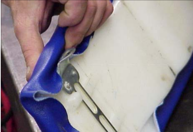
12. Work the cover in around the seat's mounting points.
