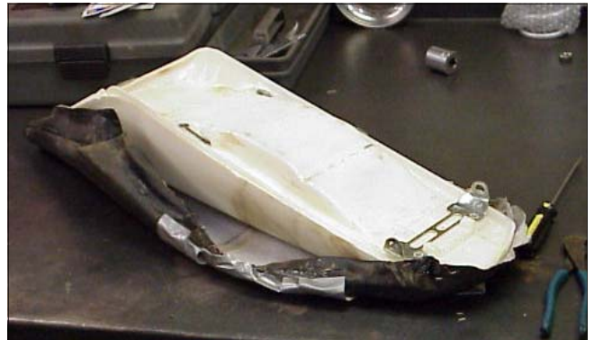
4. With all the staples out, peel the cover back
