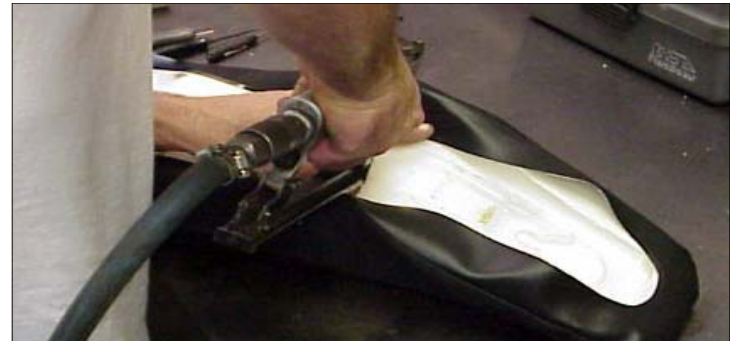
9. Then, skip round to the side of the seat at the bend. Put one in each side.
