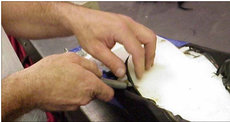
13. My WR has these mounting points in the middle of the seat. You need to trim around these.
