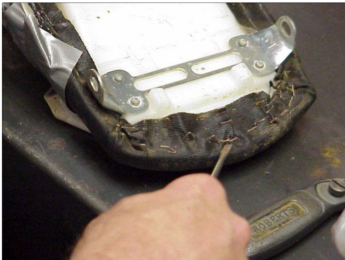
2. The first step is to remove the old seat cover. Here's Elston using a screw driver to pry the staples up.
