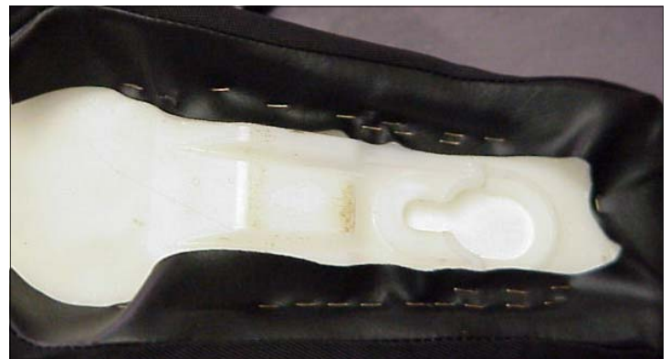
11. It's time to put some staples in the front of the seat. And continue filling in between the other staples.
