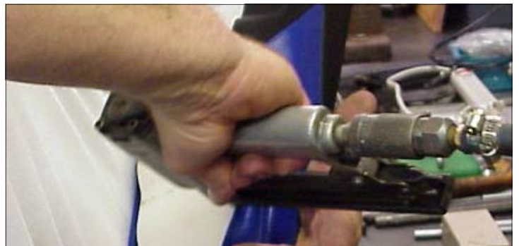
10. The next staples went in between the bend in the seat and the back. The whole time Elston was doing this, he kept pulling the seat cover tight.
