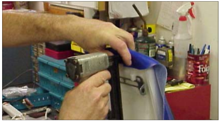
8. Elston puts in the first staple at the back of the seat.
