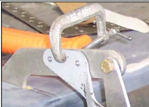
18. Install the aileron hinge to the flap bracket using AN3-6A bolts. Secure with AN365-1032 nyloc nuts and enough washer to allow the nut to tighten and show1.5-3 treads of the bolt thru the nut.
