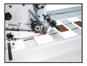
Cards are individually fed, squared and registered on the card attaching head. Pusher lugs keep the card straight throughout the attaching process. Press down rollers secure the card in place.
