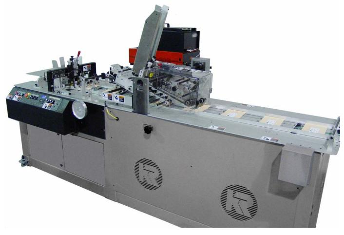
Attach cards, pharmaceutical inserts and other flat products onto various mailers and inserts using the KR 486 LR system. Designed for maximum reliability and performance, the KR 486 LR is ideally suited for applications requiring high-speed, accurate attaching of a wide variety of product.
