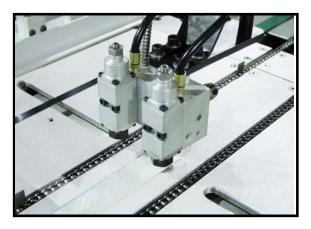
Hot melt glue heads lay down multiple strips of quick-setting hot melt glue onto the substrate.
