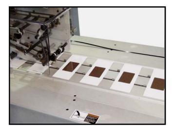
Pusher lugs on the transport and the attaching head ensure product is straight during the attaching process.
