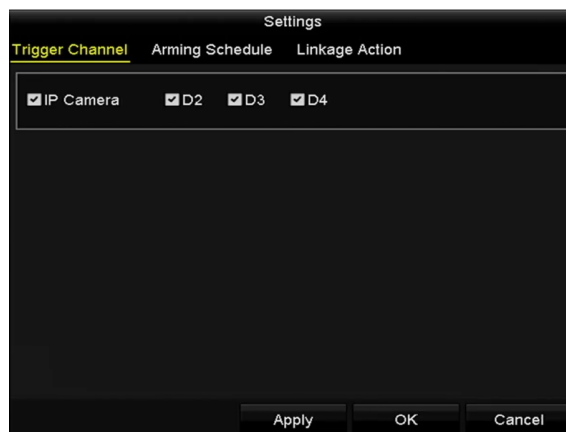
Figure 5.17 Set Trigger Camera of VCA Alarm
