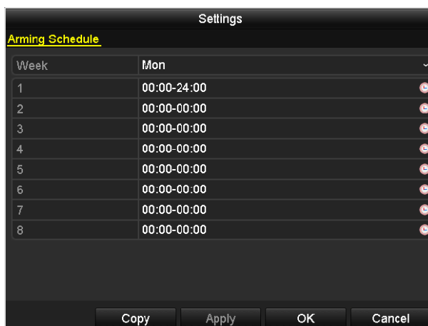
Figure 8. 17 Set Arming Schedule of Alarm Output
