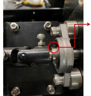
Finally, please loosen the set screw. Don't need to take down the back bearing. Then you can remove the drum.
