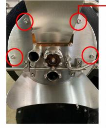
Fourthly, Loosen these bolts which are holding the front panel. Then take down the front panel.
