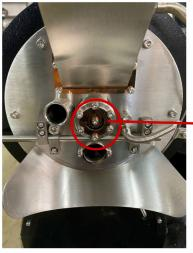
Thirdly, Loosen these 7 bolts which are holding the bearing. Take down the bearing holder and the bearing. There is a possibility that the bearing is difficult to be taken dwon, if so, please use a tool, like hammer to help with this.
