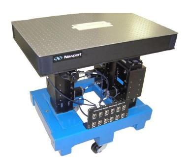
This DLS six degrees of freedom High Precision Motorized Optical Table used Newport Corporation Research Grade breadboards with a grid of M6 tapped holes. The system base was made of a welded steel frame with a powder coated finish. Frames were filled with sand to reduce the table natural frequency and provide passive damping. When in use, the table rests on four machinery feet. When in transport, the feet are retracted and casters allow for easy handling.
