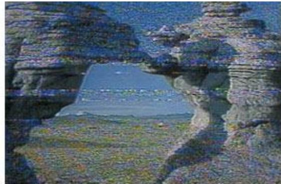
Interference caused by a thermostat
