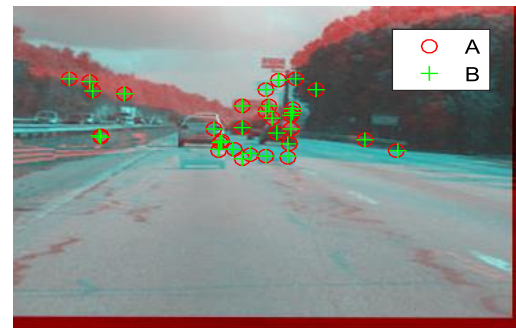
Figure 6.Overlapping of KLT features in reference frame and last frame of video
