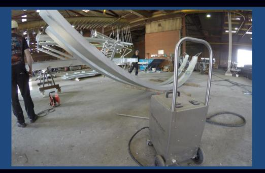
Dry ice blasting offers a completely dry and non damaging cleaning process.
