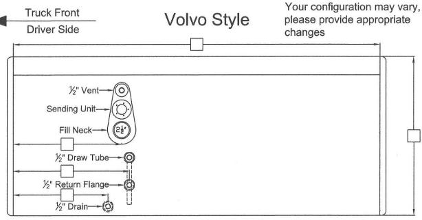
Please note: All sizes are NPTF unless otherwise noted and reference all measurements from the lateral weld seam and the end cap weld seam to the center of the fittings.
