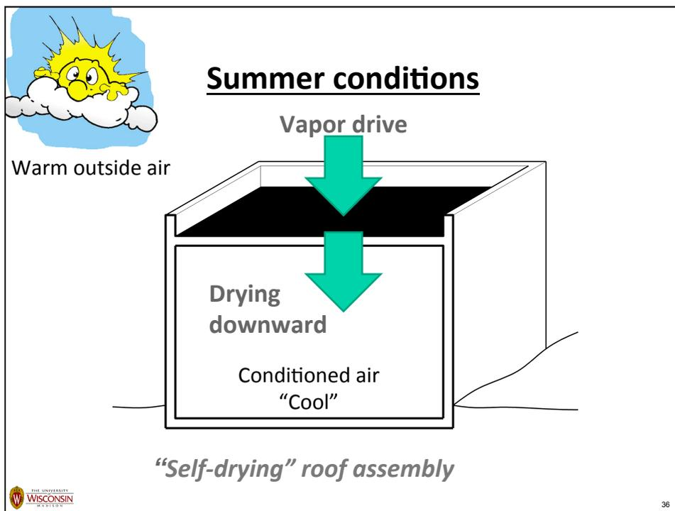
*Historically, most roof systems have effectively performed as “self-drying roofs”...*
