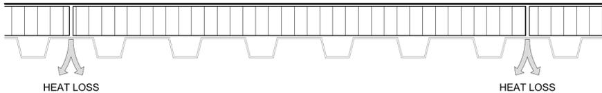
Heat loss through gaps at the joints
