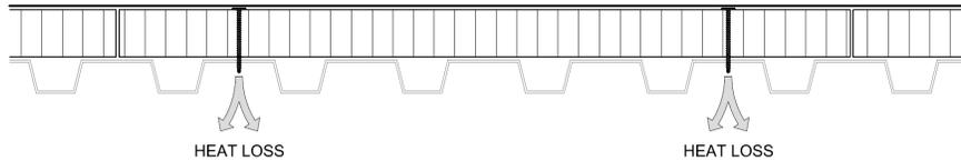
Mechanical fasteners through the cross-section of rigid board insulation can represent 3% to 8% losses in effective R-values.
