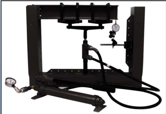
Model H-6320 Structures Test System shown with H-6320-20 wing-beam with whiffle tree option
