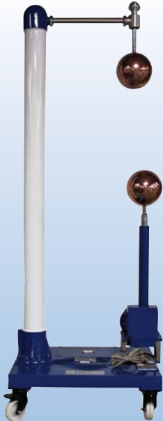
Measuring Spark Gap
