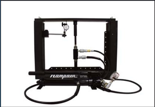
Model H-6320 Structures Test System shown with H-6320-71 flat beam assembly option
