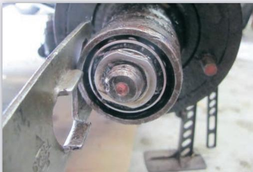
Remove the bearing for cleaning and inspection. In the photo below, notice the red grease remains in the hub cap, but the red grease in the bearing has begun to turn dark. This is a sign that the grease is working, but starting to degrade. Time for fresh grease!
