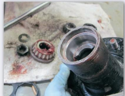
Clean all the bearings in preparation to inspect and regrease them. All the taper bearings should be clean and without cracks or excess wear. Also inspect the inner races for cracks, as well as the wheel hubs.
