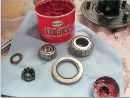
Grease well, including the inner races, and slather gobs of grease into the hub cavity, too. Refit the inner bearing, topping it off with the dust shield. The hub can then be tapped with a mallet or wood block back onto the spindle. Alternately, you can fit the dust shield over the spindle and press on the inner bearing, driving it with a sleeve tool that doesn't impact the taper bearings before fitting the hub. This is needed at times when the press fit is really nice on the spindle surface.
