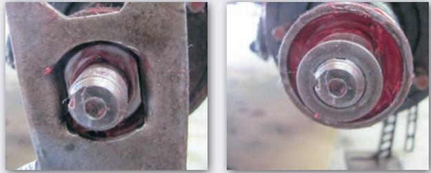
Finally, secure the spindle nut with cotter pin. Refill the hub cap with fresh grease and replace the cap.
