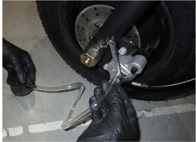
Figure 77: Bleeding the Front Brake Line
