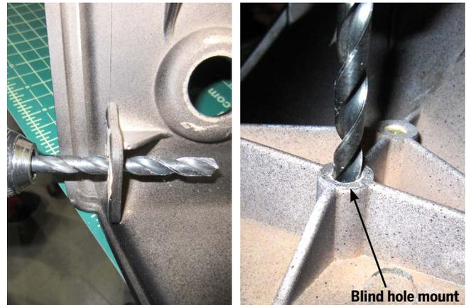
**Figure 9: Drill Out the Mounting Hole**
