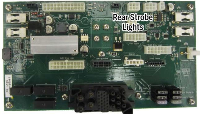
**Figure 174: Rear Strobe Light Harness to PI Board**
