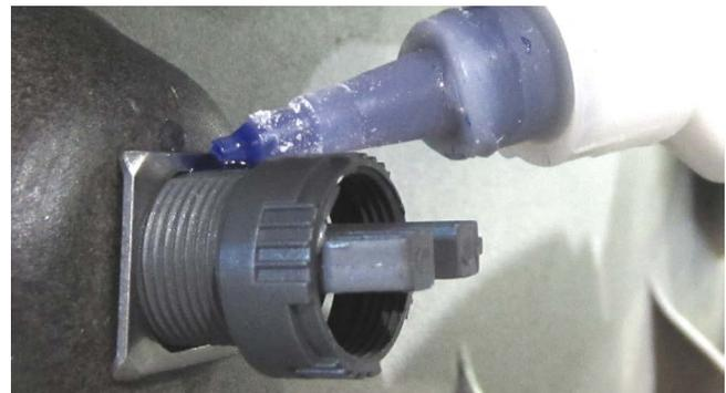
Figure 71: Apply Loctite 425
