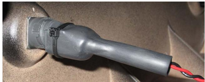
Figure 15: Rubber Protector Covering the KeyLock
