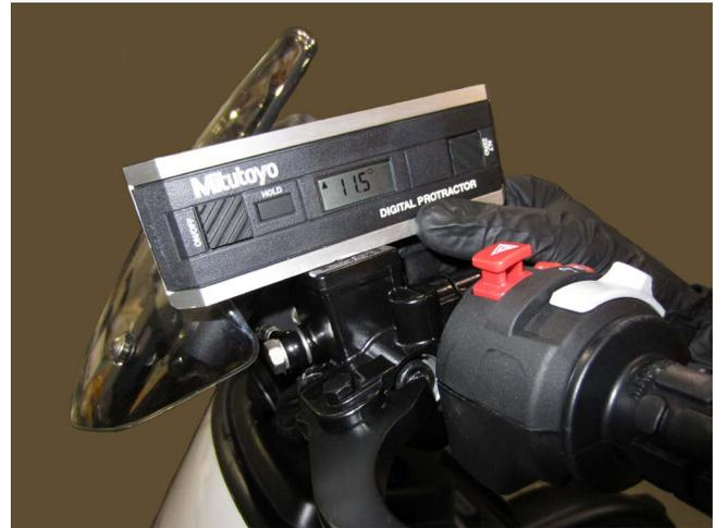
**Figure 79: Aligning the Master Cylinder**
