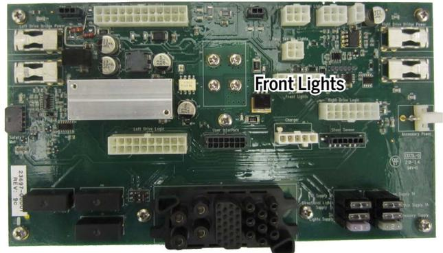
Figure 166: Light Cluster Harness to PI Board
