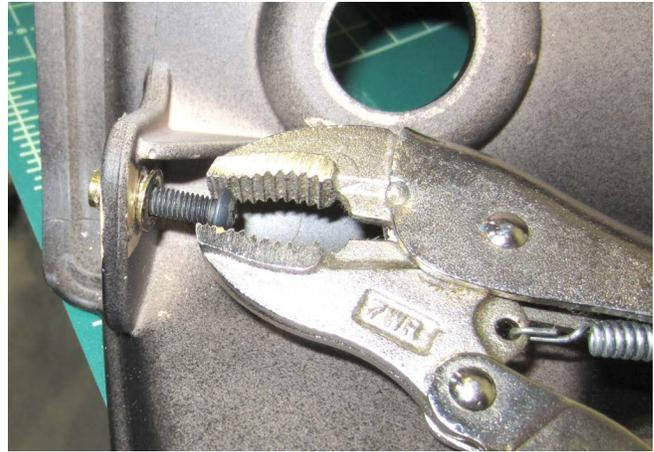
**Figure 6: Remove the Threaded Insert**
