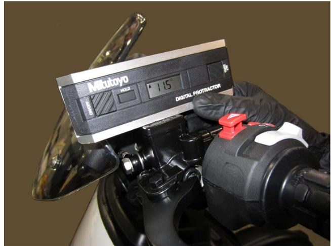
**Figure 136: Aligning the Brake Levers**
