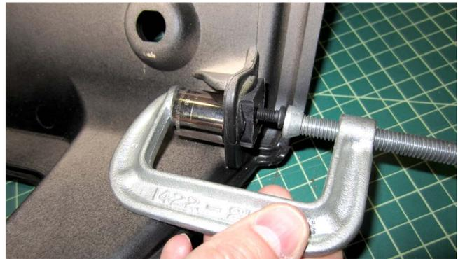
**Figure 7: Use a Clamp to Remove the Insert**
