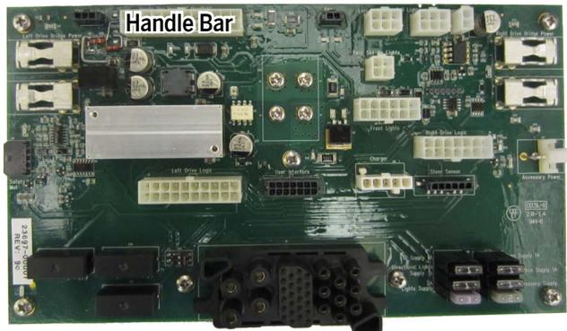
Figure 159: Handlebar Controls Harness to PI Board
