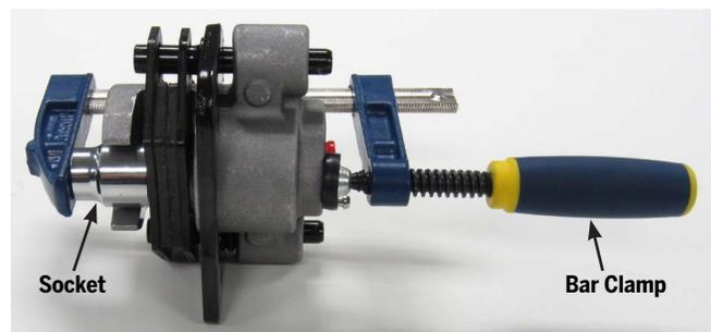
**Figure 37: Compress the Caliper**
