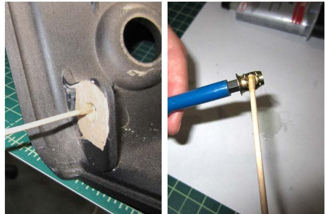
**Figure 10: Apply Epoxy**
