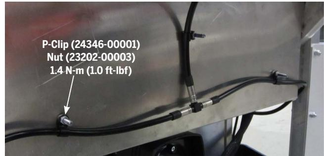
Figure 105: Brake Line P-Clips
