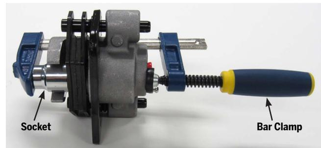
**Figure 81: Compress the Caliper**
