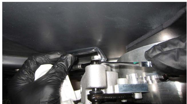
Figure 76: Draining the Rear Brake Line
