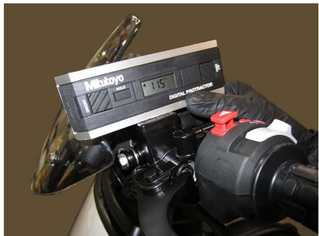
**Figure 88: Aligning the Master Cylinder**
