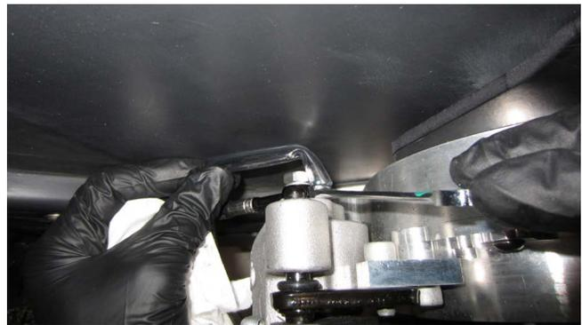
Figure 78: Bleeding the Rear Brake Line
