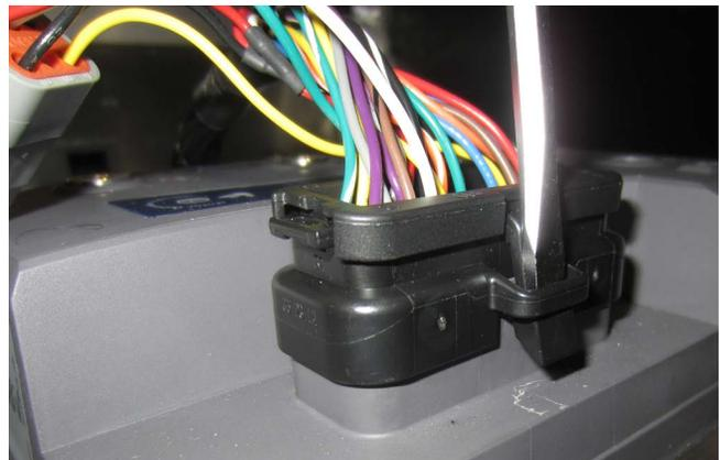
Figure 133: Removing the Harness
