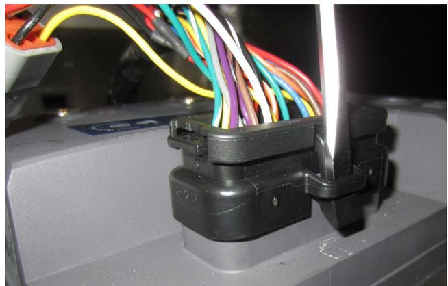
Figure 157: Drive Harness to Motor Controller
