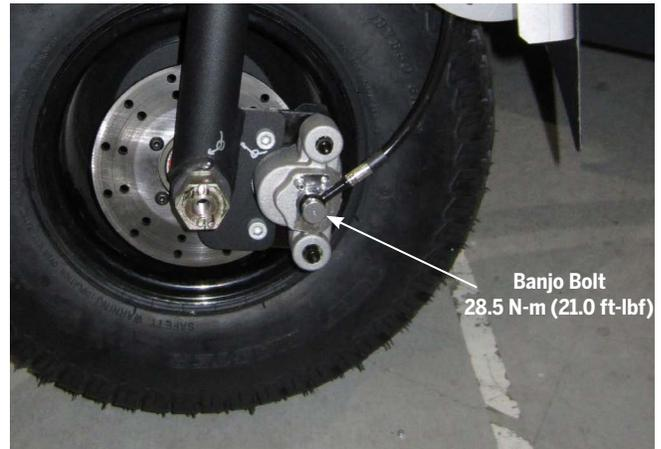
Figure 101: Front Caliper Banjo Bolt
