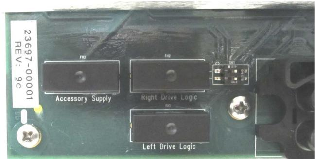
**Figure 150: Ceramic Cartridge Fuses**
