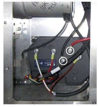
Figure 154: Motor Power Harness to Motor Controller
