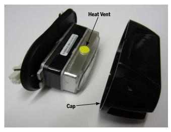
Figure 52: Heat Vent Location
