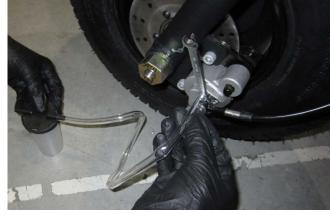
Figure 77: Bleeding the Front Brake Line
