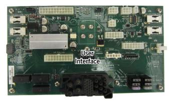
Figure 162: UI Harness to PI Board
