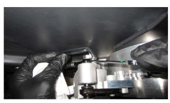
Figure 76: Draining the Rear Brake Line
