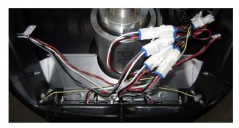
Figure 24: Light Harnesses with Cable Ties
