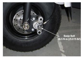
Figure 101: Front Caliper Banjo Bolt
