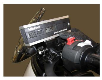
Figure 88: Aligning the Master Cylinder
