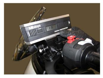
Figure 136: Aligning the Brake Levers
