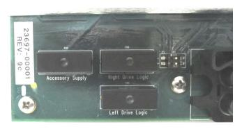
Figure 150: Ceramic Cartridge Fuses
