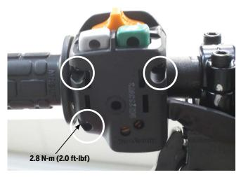
Figure 112: Control Cluster Fasteners
