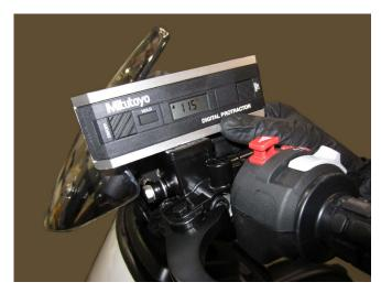
Figure 79: Aligning the Master Cylinder
