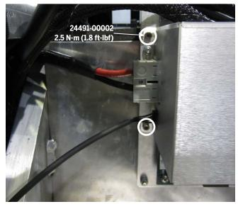
Figure 142: Left Side Fasteners
