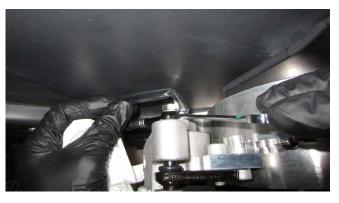
Figure 78: Bleeding the Rear Brake Line
