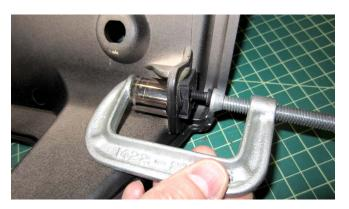
Figure 7: Use a Clamp to Remove the Insert
