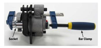
Figure 81: Compress the Caliper
