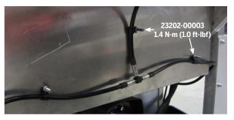
Figure 65: Brake Line P-Clips
