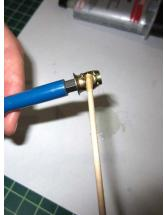
Figure 10: Apply Epoxy
