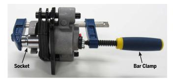
Figure 37: Compress the Caliper
