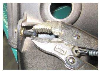
Figure 6: Remove the Threaded Insert
