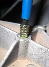
Figure 11: Install the Threaded Insert
