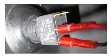
Figure 18: KeyLock Terminals
