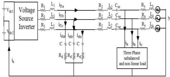
Figure 1- DSTATCOM topology to compensate Non-linear loads
