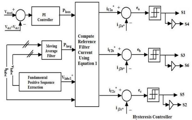
Figure 2- D-STATCOM Controller block diagram
