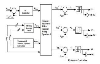
Figure 2- D-STATCOM Controller block diagram
