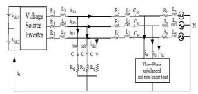
Figure 1- DSTATCOM topology to compensate Nonlinear loads
