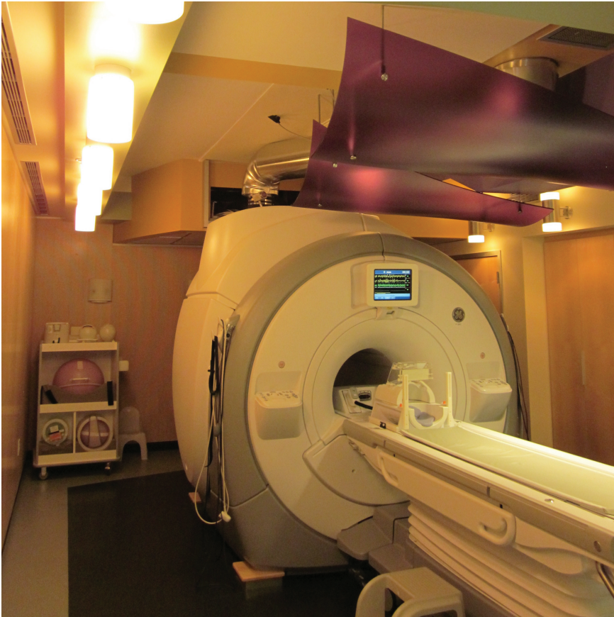
Figure 8. MRI machine. Magnetic resonance imaging systems are used to acquire both structural and functional images of the brain.
