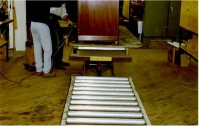
ergonomic work height. The lift was also equipped with a gravity roller conveyor bed to fit and function within the existing conveyor line. The customer is completely satisfied with this work station improvement, and worker productivity and quality have improved as a result of keeping the work more nearly within the ergonomic "power zone" of the assemblers.
