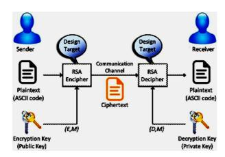
Figure 2: Encryption and decryption RSA algorithm scheme
