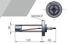
For some occasions, a quick and afford evaporation method would be required, for example making gold/ silver contact on thin films or some reference gold layer. Effusion cells will then be a too luxury and complex option as flux precision and stability will not be taken into consideration.
