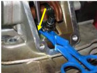
Press down on the Closing rocker to expose the retaining rings. Slight engine rotation may be required to get the rocker to move far enough to expose the retaining rings. The retaining rings are in two halves
