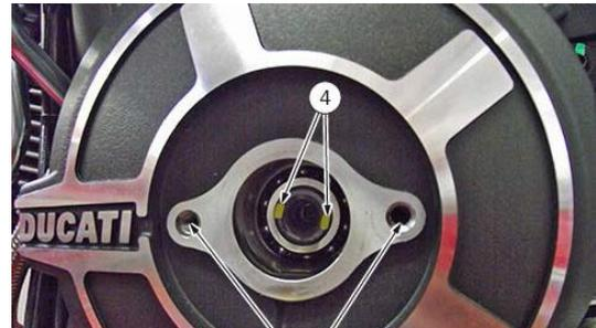
Tighten the retaining bolt snug with a 13 mm wrench.
