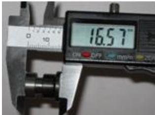
Place the Shim Measuring Tool inside the closing shim (narrow end in) and measure the overall length.
