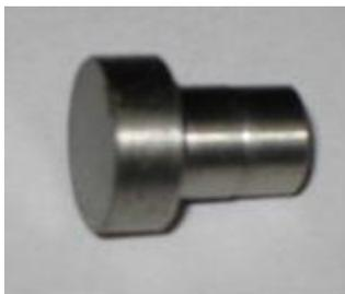
The valve shim measuring tool and the electronic caliper will be used to take the measurement. The tool sets inside of the closing shim and gives a standard 10mm addition to your measurement.
