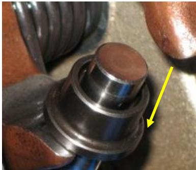
Obtain the correct shim(s) and reassemble the valve train. Slide the closing shim onto the valve stem. The wider side slides onto the valve stem first.
