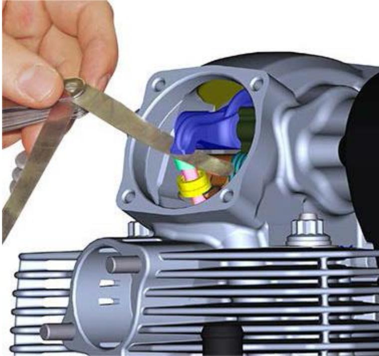
With the valve in the “rest” position, slide the feeler gauge between the opening rocker arm and the opening shim. Begin measuring using a thin gauge, ~ .05mm; proceed using thicker/thinner gauges until the gap can be determined. The correct feeling is one of slight resistance, similar to the feeling of inserting the gauge into a large book and moving it between the pages.
