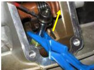
With the retaining rings removed, you can now slide the closing shim up and off the valve stem. If the shim gets "stuck" at the top of the valve stem, it is an indication the valve stem has mushroomed a bit. Some emery cloth/sandpaper is needed to remove the wide part at the top of the valve stem to provide clearance for the shim to slide off.
