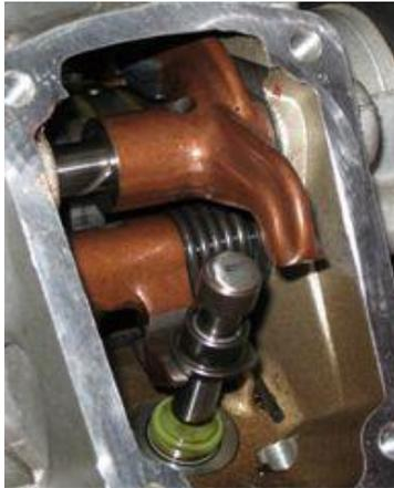
Put Opening shim onto valve stem
