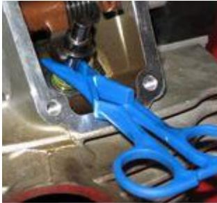
Place a clamp on the valve. In addition to having the cylinder at TDC, this is a little extra insurance to keep the valve from dropping into the cylinder.
