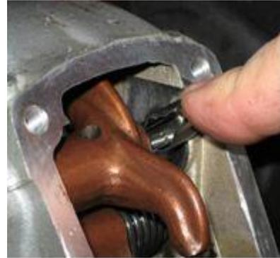
Once the rocker is in place, press the spring clip into place. Some firm pressure will be required.
