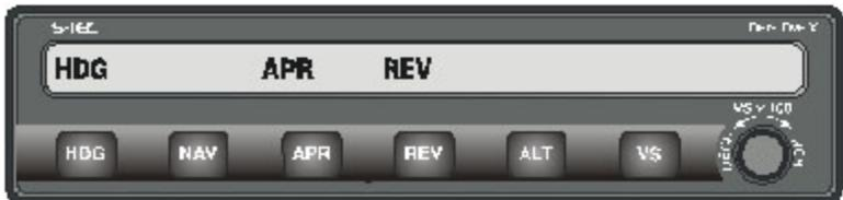
The selected heading is flown until the autopilot computes that an on-course turn must be made to minimize overshoot at the point of intercept. When the on-course turn begins, **HDG** Mode will extinguish.
