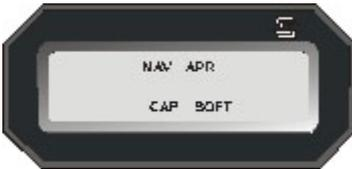
If the aircraft is equipped with a remote annunciator **NAV**, **APR**, **CAP**, and **SOFT** will be displayed.
