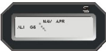
The **GS** annunciator will flash, and the **ALT** and **DSBL** annunciators will illuminate on the optional remote annunciator to indicate the **GS** Mode is disabled.
