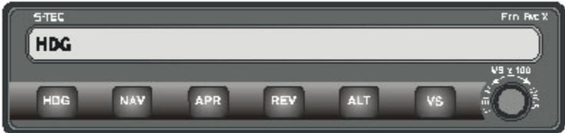
**NOTE:** When operating in the **HDG** Mode, the system is not coupled to any navigation aid. It merely flies the heading bug. It will be necessary to monitor navigation instruments for course deviation due to wind drift and wind correction angles.
