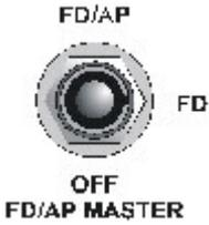
For manually controlled flight by the flight director, place the **FD/AP** master switch in the "FD" position. This disables the autopilot servos, allowing the pilot to control the aircraft to the flight director commands.
