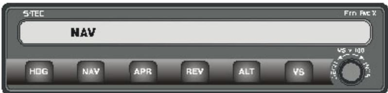
If the course needle is at full-scale deviation, the autopilot will establish a 45° intercept angle. As the aircraft approaches the selected course, the autopilot senses the closure rate and gradually shallows the intercept angle. The point at which this turn begins is variable, depending on the aircraft position and closure rate to the course. However, the turn will always begin between 100% (full-scale) needle deflection and 20% of full-scale.
