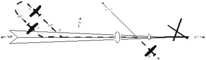
1. a. Tune navigation radio to **LOC** frequency.
