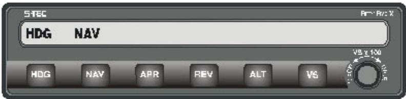
The selected heading will now be flown until the autopilot computes that an on course turn must be made to minimize overshoot at the point of intercept. At the time the on course turn begins, the **HDG** annunciator will extinguish. If using a **DG**, it is imperative that the pilot set the **HDG** bug to the selected course at this time.
