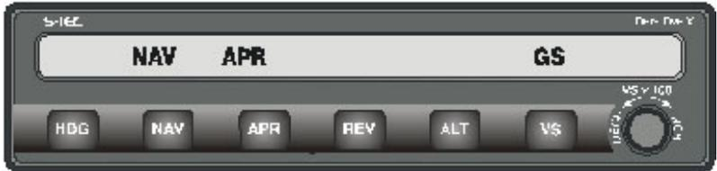
The system includes a glide-slope deviation monitor. If the aircraft strays off glide-slope centerline by 50% needle deflection, the **GS** annunciator flashes a warning. It also flashes when the **GS** flag is displayed. When this occurs, the **FAIL** annunciation will illuminate.
