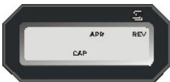
If equipped with the optional remote annunciator, the **APR**, **REV**, and **CAP** modes will be annunciated.
