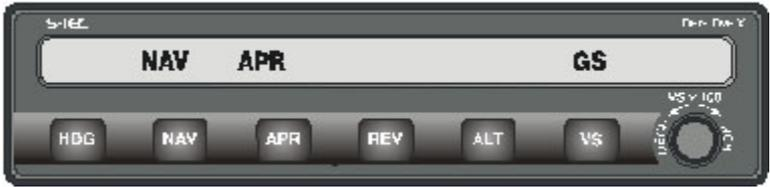
**NOTE:** If vectored to intercept the localizer too close to the glide-slope intercept point (resulting in less than 60% GS needle deviation when on course), the system will not automatically arm the glide-slope. Manual arming must be followed. (See page 4-30).
