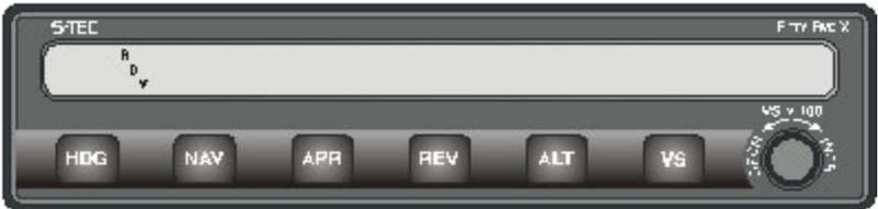
—Should a fault be detected, the **FAIL** annunciator will remain on at the conclusion of the self-test and the autopilot will not operate.
