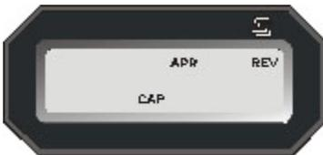
If the aircraft is equipped with the optional remote annunciator, the **APR**, **REV**, and **CAP** Modes will be annunciated.
