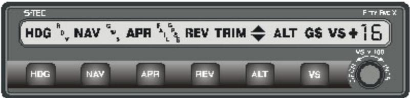
—Satisfactory completion of the **SELF-TEST** is indicated when the Ready (**RDY**) annunciator remains on at the end of the 5-second self-test.
