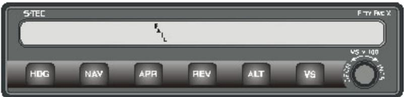
**NOTE:** If the autopilot detects the Turn Coordinator rotor speed as low or not turning, the display will remain blank and the autopilot will remain inoperable. In cold weather, the Turn Coordinator may take longer to attain proper operating speed due to temperature sensitivity. If either condition occurs, consult your dealer before use of the autopilot is attempted.
