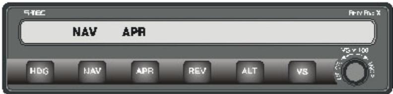
If the course needle is at full-scale deviation, the autopilot will establish a  $45^\circ$  intercept angle. As the aircraft approaches the localizer course, the autopilot senses the closure rate and gradually shallows the intercept angle. The point at which this turn begins is variable depending on the aircraft position and closure rate to the course. However, the turn will always begin between 100% (full-scale) needle deflection and 20% of full-scale.
