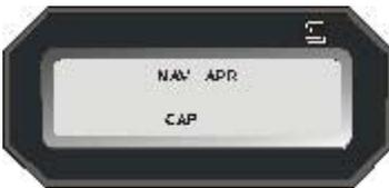
If the aircraft is equipped with the optional remote annunciator the **NAV**, **APR**, and **CAP** modes will be annunciated.
