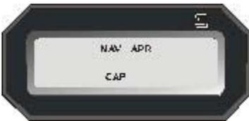
If the aircraft is equipped with the optional remote annunciator, the **NAV**, **APR**, and **CAP** modes will be annunciated.
