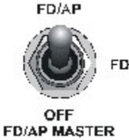
To engage the autopilot without interruption, simply place the **FD/AP** master switch in the "FD/AP" position.
