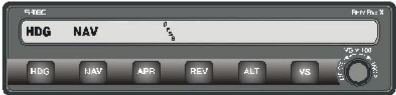
As the aircraft nears the on-course turn point, the **HDG** annunciator will extinguish.
