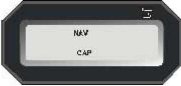
If the aircraft is equipped with an optional remote annunciator, the gain level will be indicated. **NAV** and **CAP** (Capture) Modes will be annunciated.
