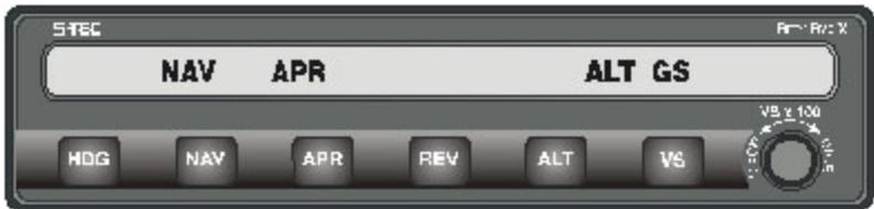
Glide-slope capture is indicated by extinguishing of the **ALT** annunciation.
