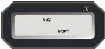
At this point, the optional remote annunciator will indicate **NAV** and **SOFT**. The **CAP** annunciator will extinguish.
