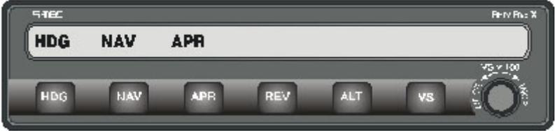
The selected heading will now be flown until the autopilot computes that an on course turn must be made to minimize overshoot at the point of intercept. At the time the on-course turn begins, the **HDG** Mode will extinguish and **you must move the heading bug to match the localizer course**.
