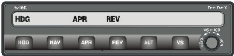
The selected heading is flown until the autopilot computes that an on-course turn must be made to minimize overshoot at the point of intercept. When the on-course turn begins, **HDG** Mode will extinguish.
