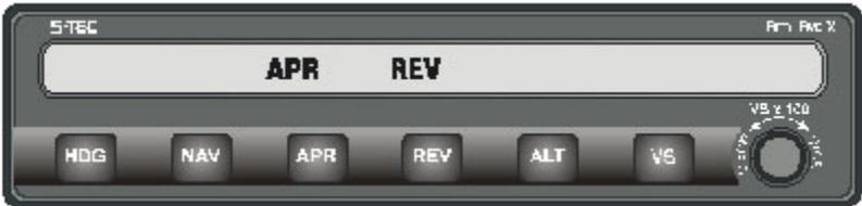
If the course needle is at full-scale deviation, the autopilot will establish a 45° intercept angle. As the aircraft approaches the localizer course, the autopilot senses the closure rate and gradually shallows the intercept angle. The point that this turn begins is variable depending on the aircraft position and closure rate to the course. However, the turn will always begin between 100% (full-scale) needle deflection and 20% of full-scale.
