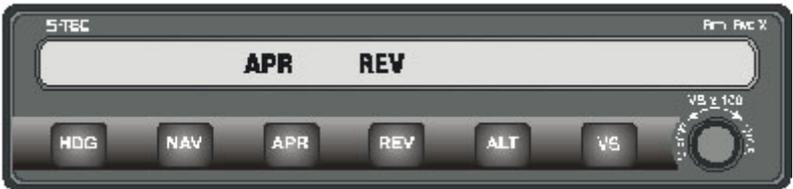
If the course needle is at full-scale deviation, the autopilot will establish a 45° intercept angle. As the localizer course is approached, the autopilot senses the closure rate and gradually shallows the intercept angle. The inbound turning point is variable, depending on aircraft position and closure rate to the course. However, the turn will always begin between 100% (full-scale) needle deflection and 20% of full-scale.
