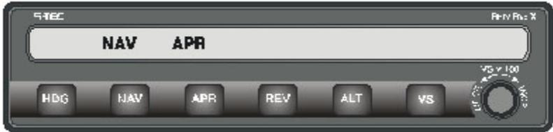
If the course needle is at full-scale deviation, the autopilot will establish a  $45^\circ$  intercept angle. As the aircraft approaches the localizer course, the autopilot senses the closure rate, and gradually shallows the intercept angle. The point that this turn begins is variable depending on the aircraft position and closure rate to the course. However, the turn will always begin between 100% (full-scale) needle deflection and 20% of full-scale.
