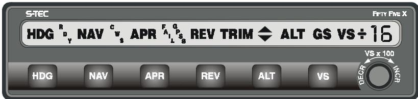
The Roll Computer receives select input signals from the Directional Gyro (**DG**) or Horizontal Situation Indicator (**HSI**), Very High Frequency Omni-directional Radio (**VOR**), Localizer (**LOC**) or Global Positioning System (**GPS**), Deviation Indicators, and the Turn Coordinator. It then computes roll servo commands for stabilization, turns, navigation intercepts, and tracking.
