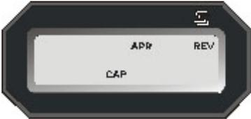
If the aircraft is equipped with an optional remote annunciator, the **APR**, **REV**, and **CAP** modes will be annunciated.
