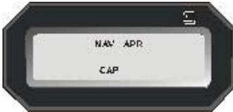
If the aircraft is equipped with the optional remote annunciator, the **NAV**, **APR**, and **CAP** modes will be displayed.
