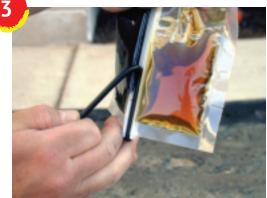
Remove the resin pouch and lay flat. Grasping the pouch on either end, gently pull the two sides apart until the separator tube pops up. Pull the tube out moving from top to bottom.
