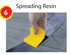
Work the Eli-Flex into the surface using a spatula or any other flat-edged tool. Working time is approximately 20-30 minutes. After approximately 45 minutes the resin will gel, and after 120 min it will set. It is now ready for belt operation, but will take 8-10 hrs to reach full strength.
