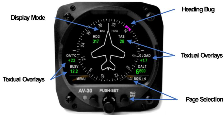
Figure 18 – Basic DG Mode User Interface
