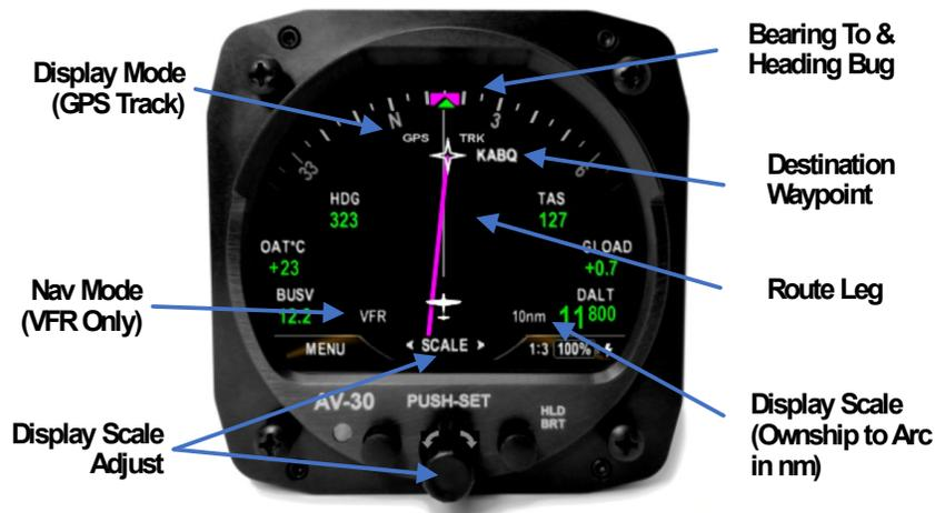
Figure 20 – GPS ARC Mode
