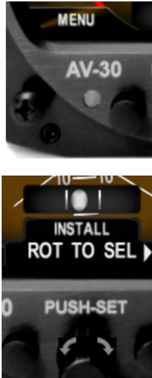
Figure 39 – Installation Menu Access
