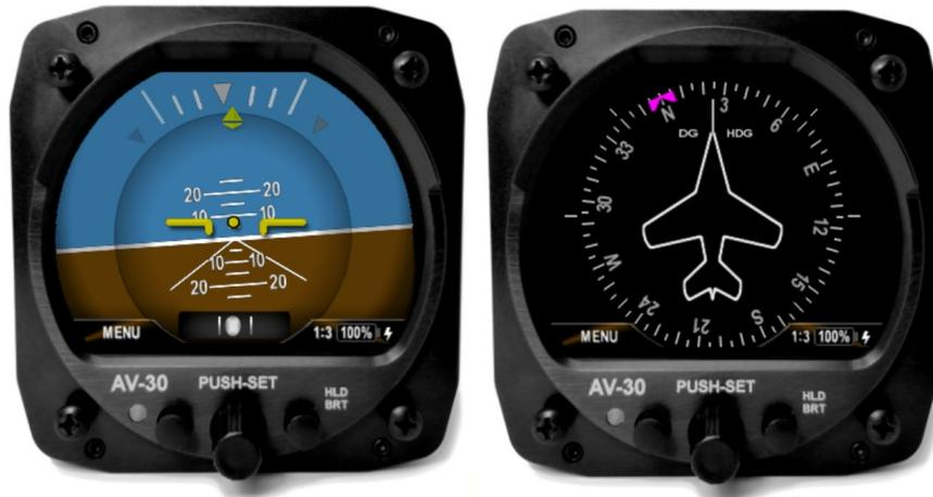
Figure 1 - AV-30-E Multi Mode AI/DG – Basic Display
