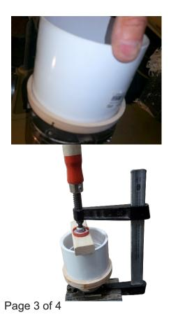
Mark OD of PVC on flattened face of block with compass, dividers, or by centering coupler to spinning wood block and marking with pencil. Using 3/16" parting tool, initiate cut, stopping lathe often, test fit and adjust and turn the groove for coupler. Bore approximately 3/8" to 1/2" deep. Reduce turning pressure, keep firm on tool rest (no bounce), tool sharp and make sure final cut is level and true.
