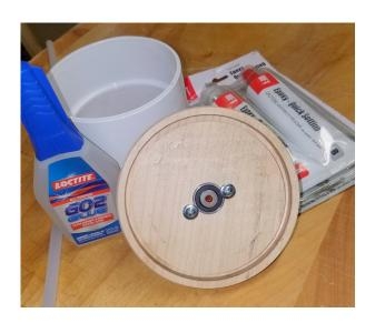
I believe the tenon/dovetail is the most economical, "frugal" and efficient way of attaching. It is time efficient also, you remove your workpiece from the 4 jaw chuck, and then attach your vacuum coupler.
