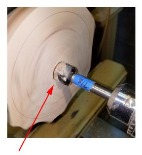
Use a 7/8" dia. Forstner bit using drill chuck in tail stock to bore the depth of the bearing thickness, 1/4". Then a 3/4" Forstner bit, through bore to allow clearance for coupling. Drill press could also be utilized, make sure bore is centered.
