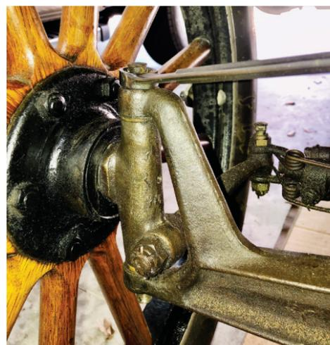
After adjusting the spindle bolt, turn the steering wheel to be sure of free movement, as a spindle bolt that is too tight can bind the spindle and make steering difficult.
