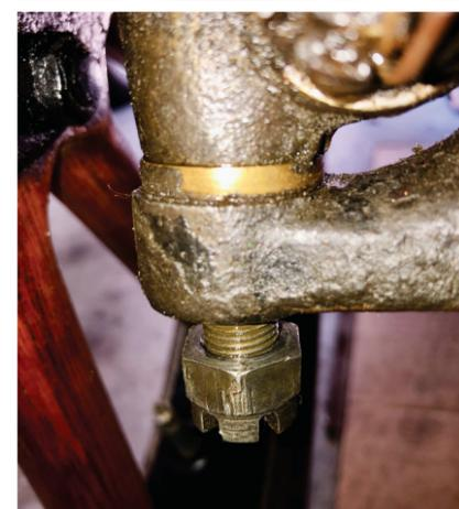
Finally, hold the upper head of the spindle bolt that has been adjusted, in place, with one wrench. At the same time, tighten the castle lock nut firmly with another wrench and align the cotter hole. Replace that safety cotter pin to secure and lock the nut.
