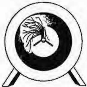
Tracer will lie down in flight and fluff out on impact at target.
