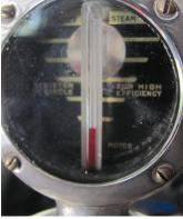
After the test run I measured the temperature of the upper tank with the engine still running at idle speed; the reading was 183.5°. The normal ideal for an internal combustion engine is in the 180° range. The Motometer matched the efficiency reading, too.
